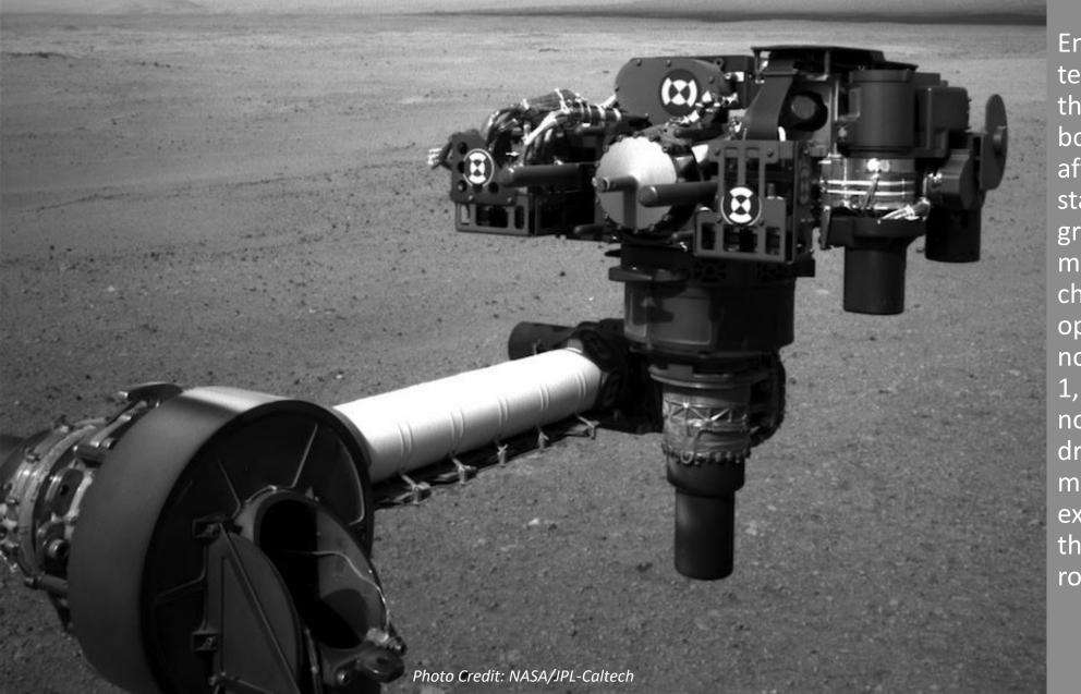
Engineers have started testing a new way to use the Curiosity rover's drill to bore into Martian rocks after a motor in the device stalled late last year, but ground teams are still months away from the first chance to resume drilling operations. The rover has not used its drill since Dec. 1, 2016, when engineers noticed a problem with the drill feed mechanism, a motor which is supposed to extend the drill bit to touch the surface of Martian rocks.
